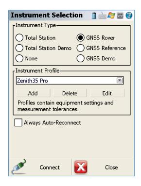
To ensure that measured heights are computed correctly, it is important to define the receiver type. At the *Antenna Height* panel, choose the Model as **Zenith35 Pro**. The Measured Height is the default length of the telescopic pole.
