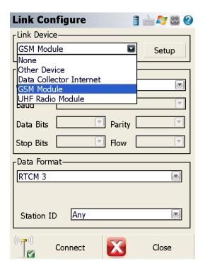
Set the Data Format with the required RTK base message type. When selecting **GSM Module** or **Data Collector Internet**, tap Setup to define the NTRIP parameters. Once an internet connection is established, a suitable mountpoint can be selected.
