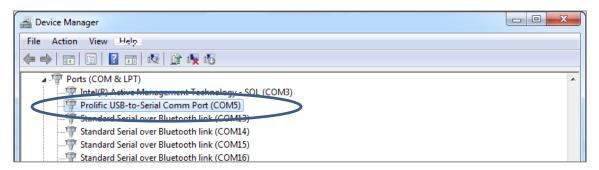
The COM Port defaults are Baudrate 115`200, 8 databits, 1 Stopbit, Parity None.
