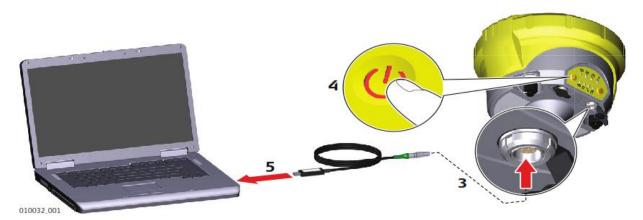
After the successful installation your hardware can be used as a mass storage device. Files can now be uploaded and/or downloaded to the Zenith35 Pro.
