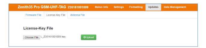
The licence key file can be installed onto the receiver by using GeoMax Z35WebManager. With the receiver connected to the GeoMax Z35WebManager, select option  $Updates \rightarrow License$ -Key File. Choose the key file (for example  $L_xxx.key$  where xxx is the receiver serial number) and click Upload. A confirmation message will be shown once the option has been activated.
